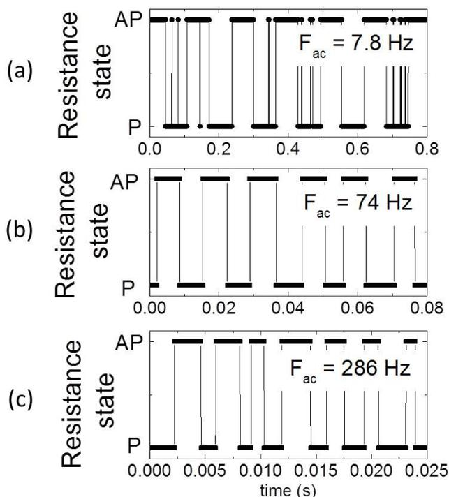
Fig. 1. Resistance as a function of time of a superparamagnetic tunnel junction driven by a periodic square wave current of fixed amplitude  $200 \mu\text{A}$  and varying frequency. When the frequency of the injected current matches the frequency of the stochastic nano-oscillator, noise-enhanced synchronization occurs (panel b).
