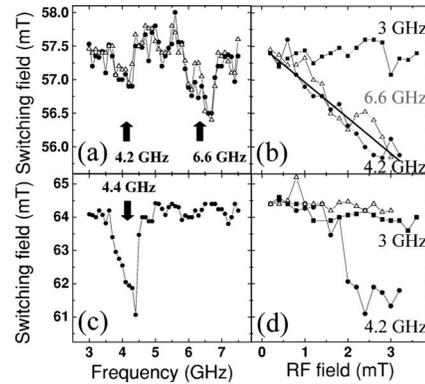
FIG. 3. (a) Average of  $up^{NoP}$  ( $\triangle$ ) and average of  $dn^P$  ( $\bullet$ ) vs frequency with a 2.2 mT microwave field. (b) Average of  $up^{NoP}$  and  $dn^P$  vs  $H_{MW}$  at 3 GHz  $\blacksquare$ , 4.2 GHz  $\bullet$ , 6.6 GHz  $\triangle$ . The line is the fit to the model. (c)  $\bullet$ :  $up^P$  vs frequency with a 2.2 mT microwave field. (d)  $up^P$  vs  $H_{MW}$  at 3 GHz  $\blacksquare$ , 4.2 GHz  $\bullet$ , 6.6 GHz  $\triangle$ .
