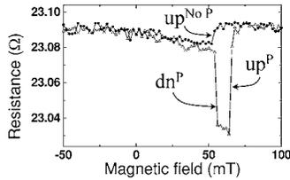
FIG. 2. Resistance vs static magnetic field  $H$  curves measured at room temperature. Here  $H$  is parallel to the strip's longest dimension and slowly swept from  $-100$  to  $+100$  mT. With the same sample, two behaviors  $\bullet$  or  $\triangle$  can be observed.
