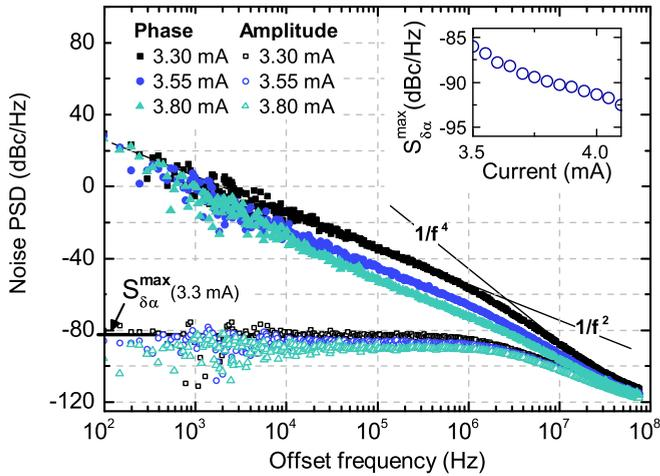
FIG. 2. (Color online) Amplitude (empty dots) and phase (full dots) noise PSD at  $H_{\perp} = 4.4$  kOe obtained for different values of current  $I$  (in mA): 3.30 (black squares), 3.55 (blue circles), and 3.80 (green triangles) that correspond respectively to STNO output voltage integrated power of 11, 15, and 23 nW. Inset: Amplitude noise maximum level vs current  $I$ .
