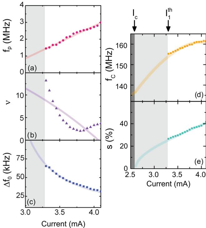
FIG. 4. (Color online) Response-to-noise parameters versus current  $f_p$  (a),  $\nu$  (b) and  $\Delta f_0$  (c). Vortex dynamic features versus current: carrier frequency (d) and normalized orbit radius (e) for  $H_{\perp} = 4.4$  kOe. The symbols correspond to measurement data, and the solid lines to theoretical curves.
