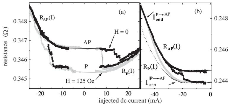
Fig. 1. Resistance vs. dc current: (a) sample 1 for  $H_{\text{appl}} = 0$  (black) and  $H_{\text{appl}} = 125$  Oe (gray); (b) sample 2 for  $H_{\text{appl}} = 0$  (black),  $H_{\text{appl}} = +500$  Oe (gray) and  $H_{\text{appl}} = +5000$  Oe (dotted line).
