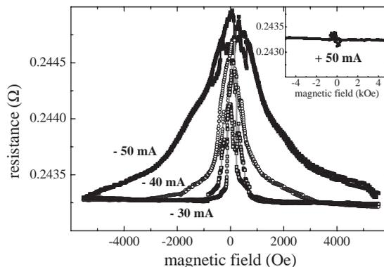
Fig. 3. Resistance vs. applied magnetic field in sample 2 for  $I = -50, -40,$  and  $-30$  mA. For clarity, the curves have been shifted vertically to have the same high field baseline. inset:  $R(H)$  for  $I = +50$  mA.
